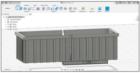
Photo 1; the body in 2 halves which has been designed to just slot together with the use of 4 x 4mm dowels.
