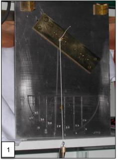
My first project was a "Capuchin Dial "made on a bit of scrap aluminium plate rescued from a cover of a piece of dead equipment. I spent a Christmas with a ruler and a scriber scratching each hour line into the plate. Numbers were created by using number punches. It was pretty crude, but I had to work with what few tools I had. I am not sure where the original dial is now, but here (**Picture 1**) is a
